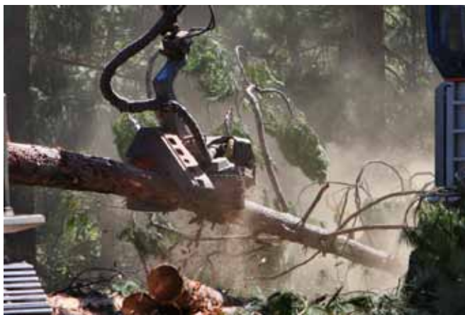
De-limbering machine works on timber. Photo by Velo Steve.
